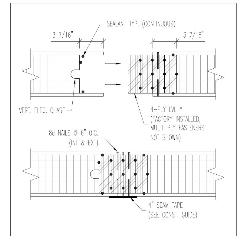
\* MULTI-PLY LUMBER TO BE GLUED, SEALED & NAILED TOGETHER AT FACTORY.
