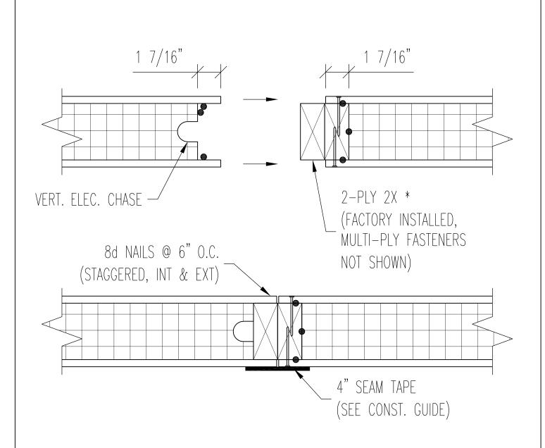
\* MULTI-PLY LUMBER TO BE GLUED, SEALED & NAILED TOGETHER AT FACTORY.
