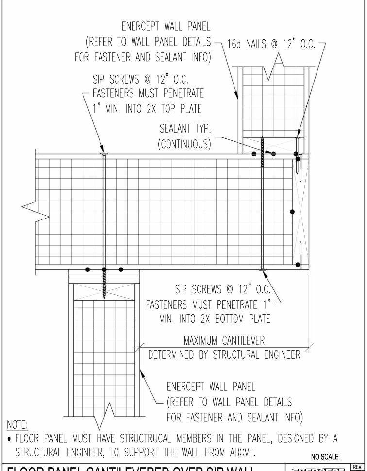
FLOOR PANEL CANTILEVERED OVER SIP WALL SUPPORTING SIP WALL ABOVE
