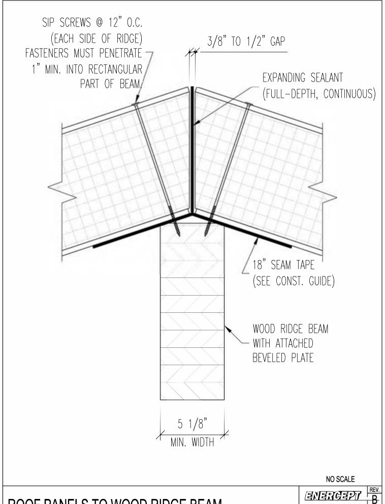
ROOF PANELS TO WOOD RIDGE BEAM
