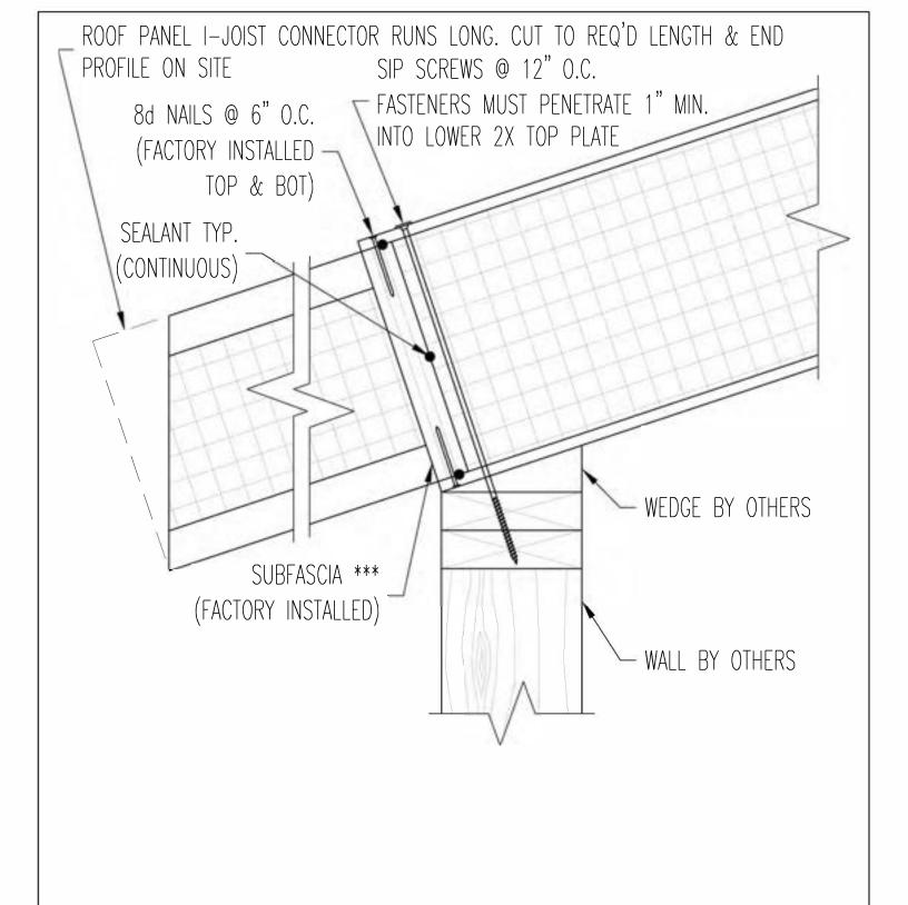
\*\*\* SUBFACIA INSTALLED IS BASED ON ROOF PANEL THICKNESS AND/OR STRUCTURAL REQUIREMENTS. ENERCEPT MAY INSTALL DIMENSIONAL 2X LUMBER, RIMBOARD, OR LVL. NO SCALE
