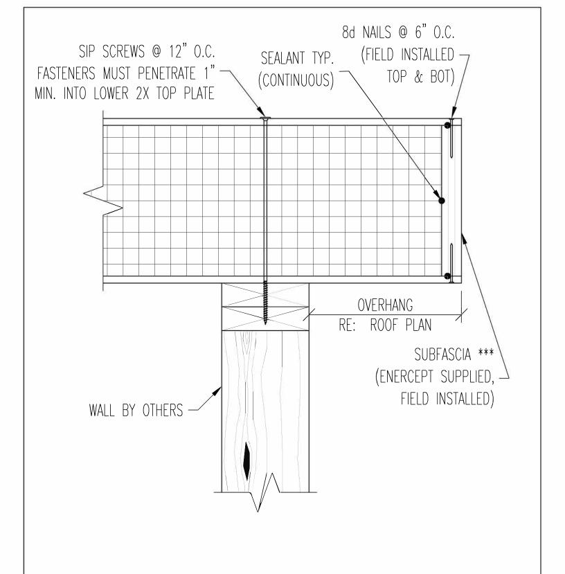
\*\*\*\* SUBFACIA SUPPLIED IS BASED ON ROOF PANEL THICKNESS AND/OR STRUCTURAL REQUIREMENTS. ENERCEPT MAY SUPPLY DIMENSIONAL 2X LUMBER, RIMBOARD, OR LVL. NO SCALE
