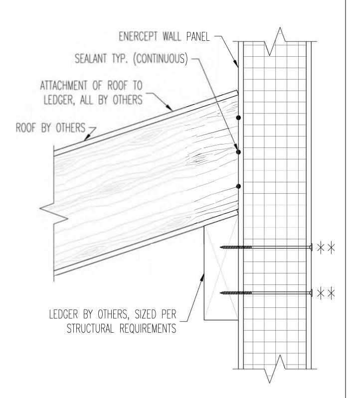
NOTE: ATTACHMENT OF LEDGER TO EXTERIOR OF WALL PANEL BY OTHERS.
