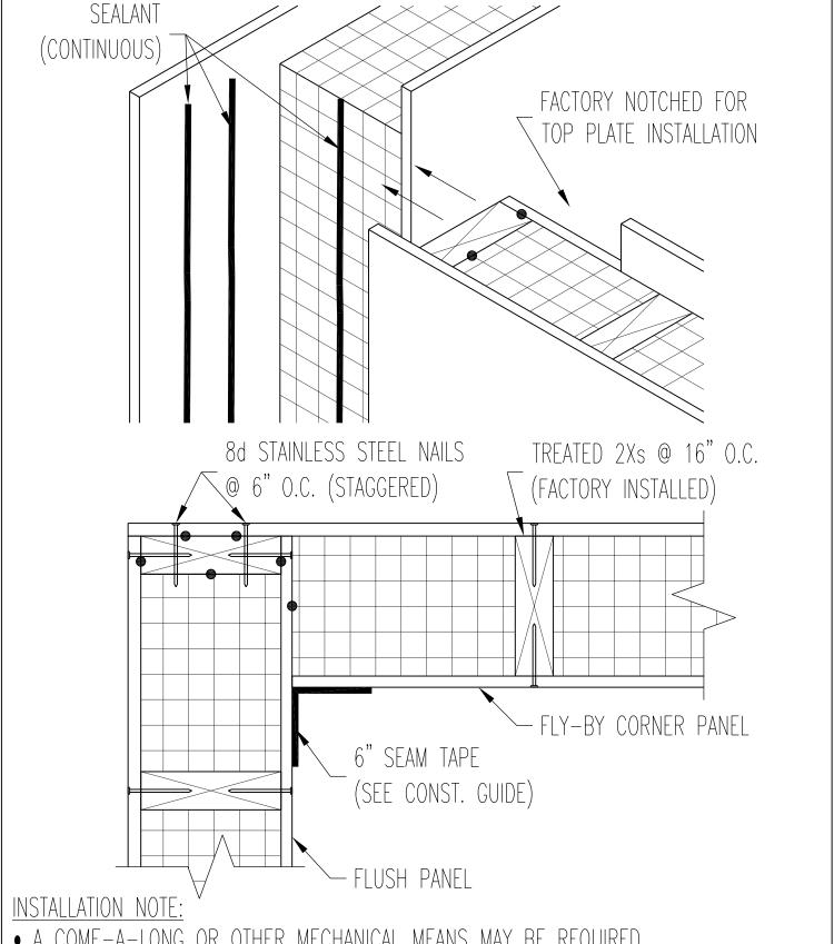
• A COME-A-LONG OR OTHER MECHANICAL MEANS MAY BE REQUIRED TO PULL PANELS TOGETHER.
