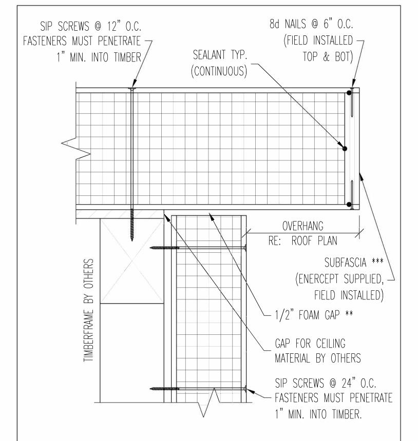
\*\*\* SUBFACIA SUPPLIED IS BASED ON ROOF PANEL THICKNESS AND/OR STRUCTURAL REQUIREMENTS. ENERCEPT MAY SUPPLY DIMENSIONAL 2X LUMBER, RIMBOARD, OR LVL.
