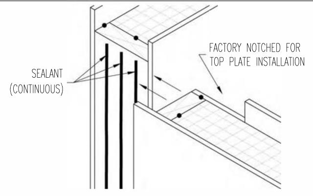
SIP SCREWS @ 24" O.C. - FASTENERS MUST PENETRATE 1" MIN. INTO 2X END CAP
