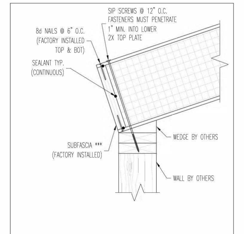
\*\*\* SUBFACIA INSTALLED IS BASED ON ROOF PANEL THICKNESS AND/OR STRUCTURAL REQUIREMENTS. ENERCEPT MAY INSTALL DIMENSIONAL 2X LUMBER, RIMBOARD, OR LVL. NO SCALE
