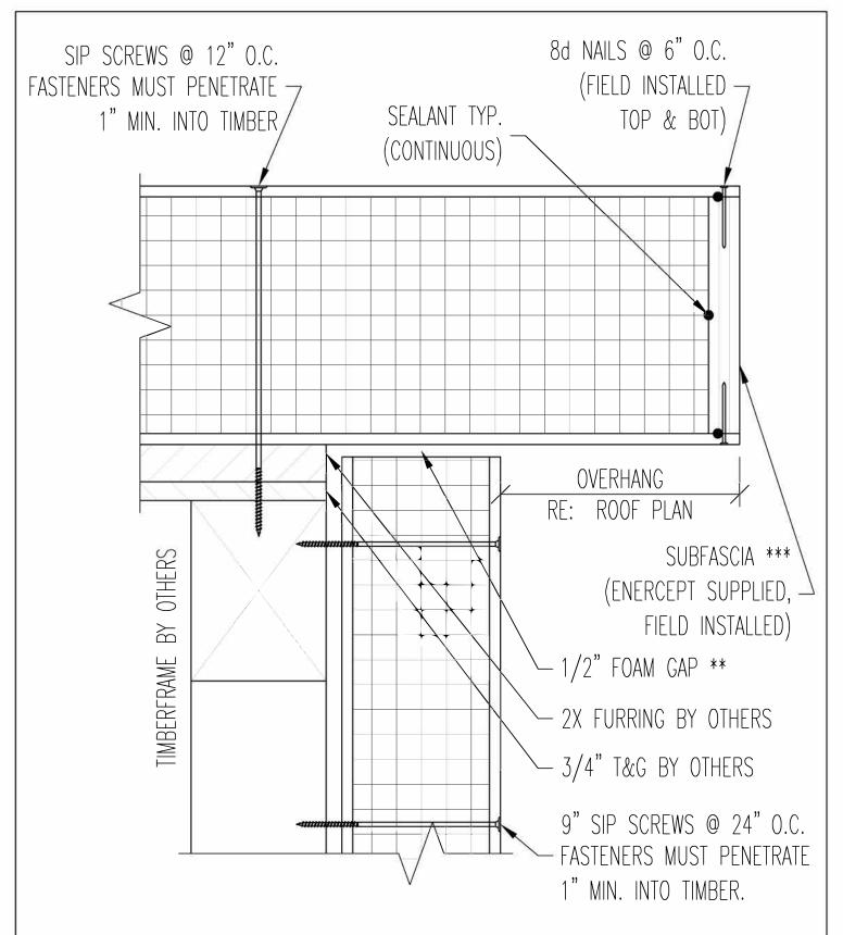
\*\*\* SUBFACIA SUPPLIED IS BASED ON ROOF PANEL THICKNESS AND/OR STRUCTURAL REQUIREMENTS. ENERCEPT MAY SUPPLY DIMENSIONAL 2X LUMBER, RIMBOARD, OR LVL. NO SCALE
