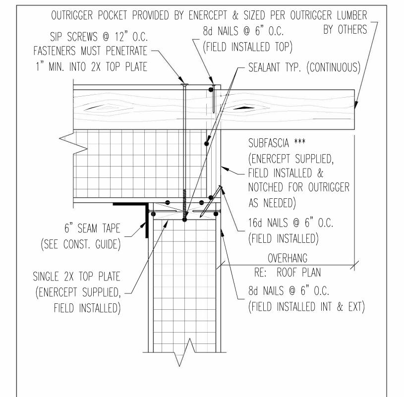
• WALL PANELS AT GABLE ENDS DO NOT RECEIVE A CAP PLATE OVER THE FULLY RECESSED TOP PLATE UNLESS NOTED OTHERWISE.
