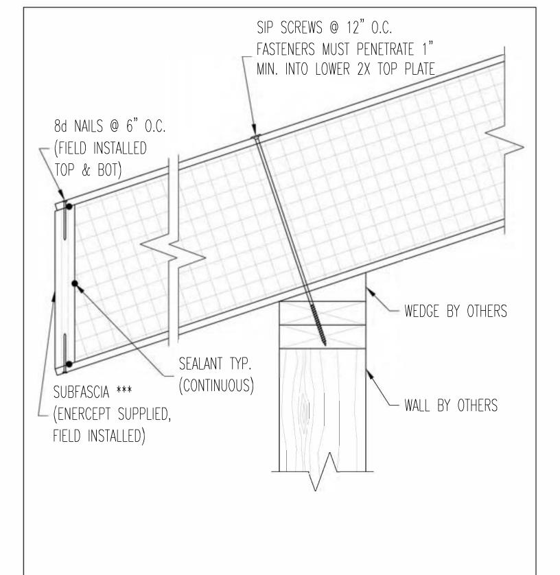
\*\*\* SUBFACIA SUPPLIED IS BASED ON ROOF PANEL THICKNESS AND/OR STRUCTURAL REQUIREMENTS. ENERCEPT MAY SUPPLY DIMENSIONAL 2X LUMBER, RIMBOARD, OR LVL. NO SCALE
