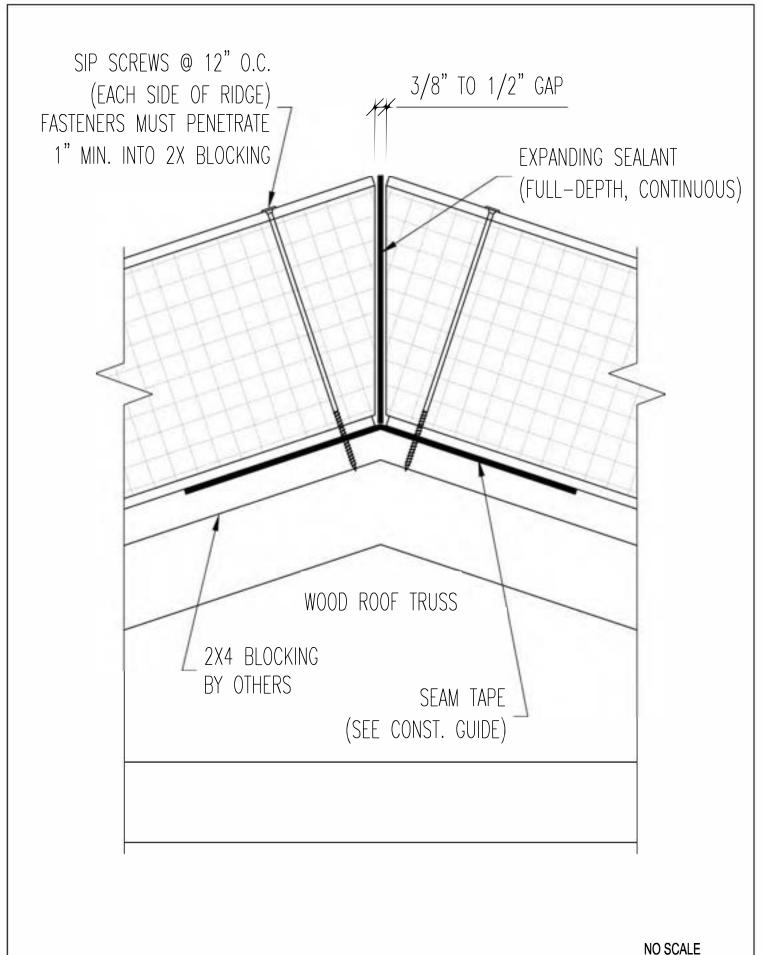
ROOF PANEL TO WOOD ROOF TRUSS WITH TOP 2X BLOCKING, AT RIDGE
