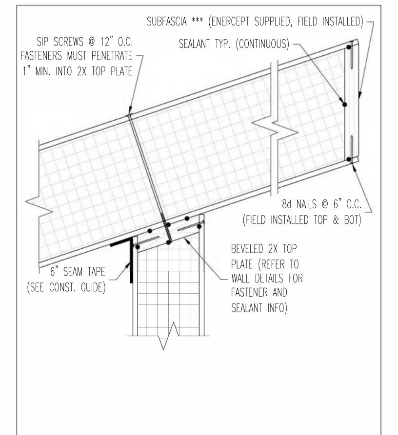
ROOF PANEL, PLUMB CUT, PANEL OVERHANG, BEVELED WALL PANEL AT UPPER EAVE
