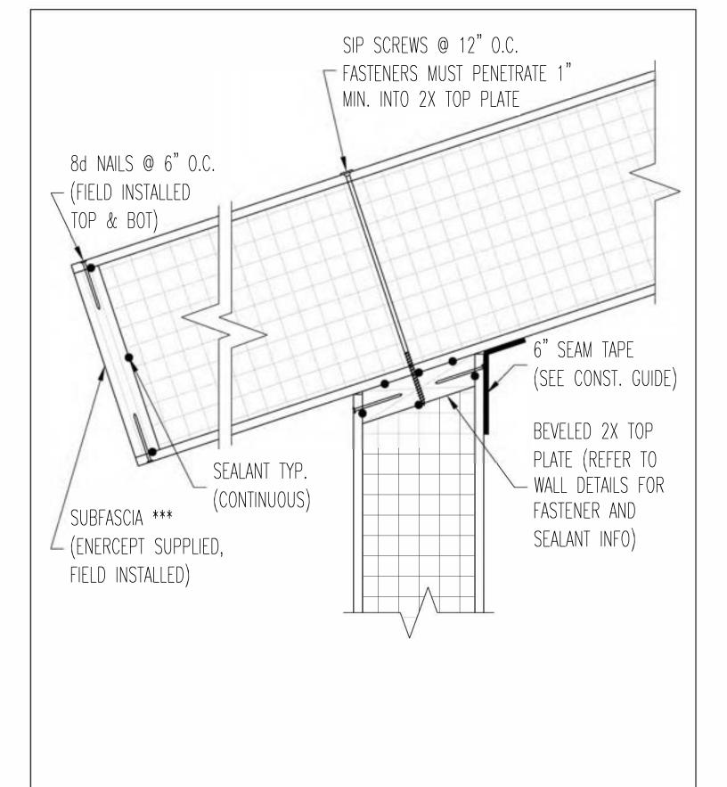
ROOF PANEL, SQUARE CUT, PANEL OVERHANG, BEVELED WALL PANEL AT EAVE
