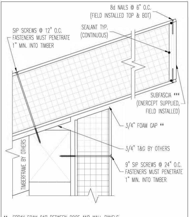
\*\*\* SUBFACIA SUPPLIED IS BASED ON ROOF PANEL THICKNESS AND/OR STRUCTURAL REQUIREMENTS. ENERCEPT MAY SUPPLY DIMENSIONAL 2X LUMBER, RIMBOARD, OR LVL. NO SCALE
