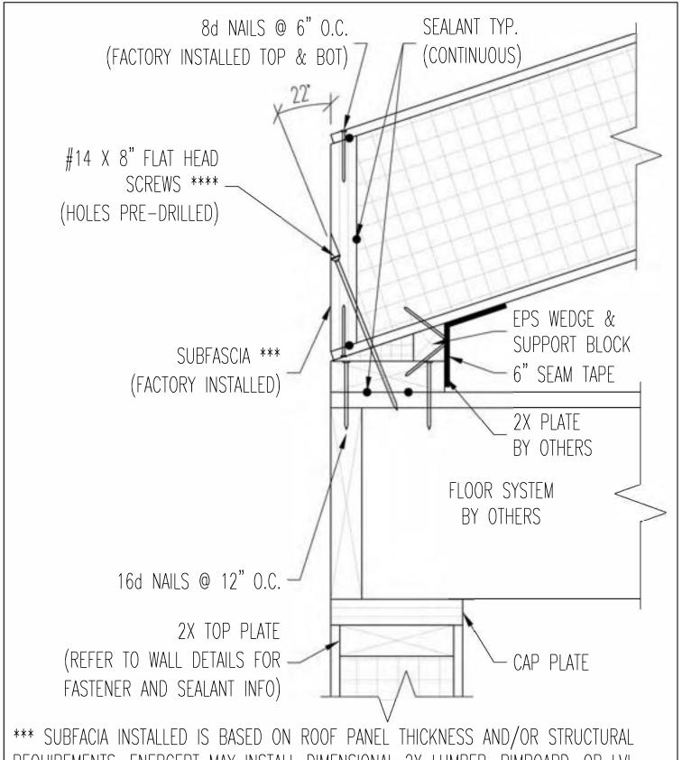
\*\*\* SUBFACIA INSTALLED IS BASED ON ROOF PANEL THICKNESS AND/OR STRUCTURAL REQUIREMENTS. ENERCEPT MAY INSTALL DIMENSIONAL 2X LUMBER, RIMBOARD, OR LVL.
