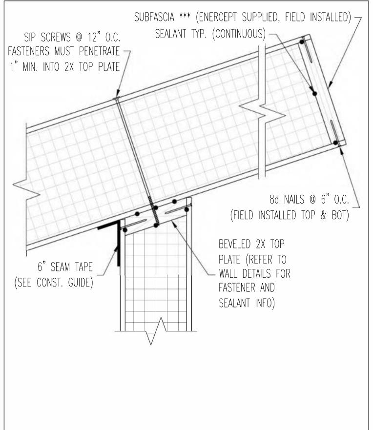
ROOF PANEL, SQUARE CUT, PANEL OVERHANG, BEVELED WALL PANEL AT UPPER EAVE
