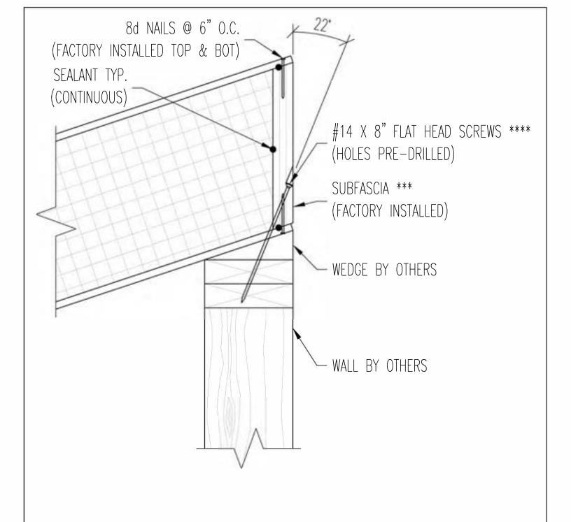
\*\*\* SUBFACIA INSTALLED IS BASED ON ROOF PANEL THICKNESS AND/OR STRUCTURAL REQUIREMENTS. ENERCEPT MAY INSTALL DIMENSIONAL 2X LUMBER, RIMBOARD, OR LVL.
