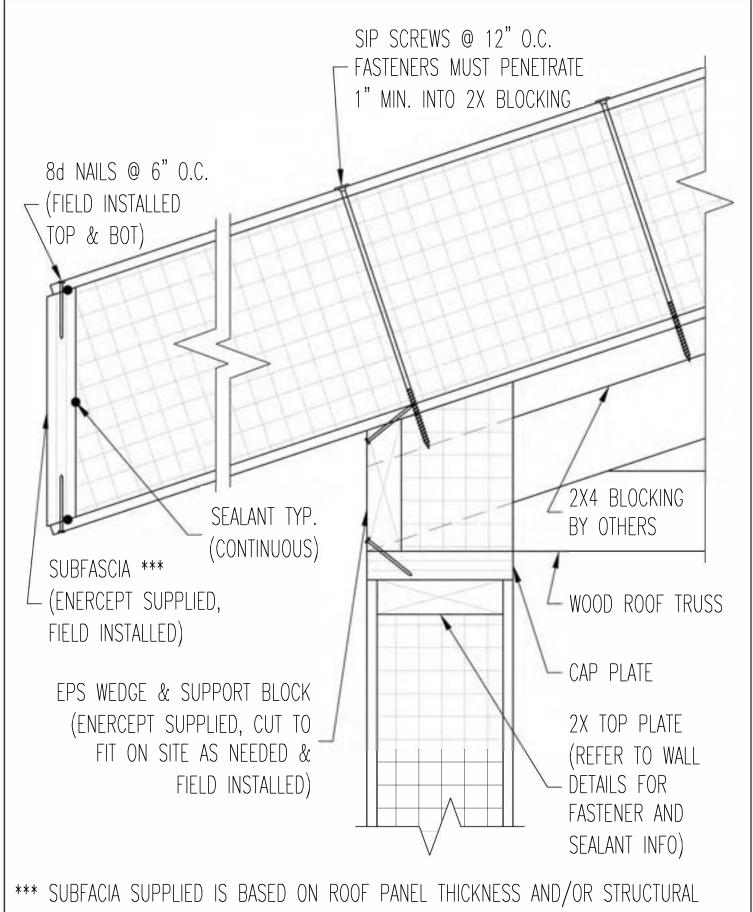
\*\*\* SUBFACIA SUPPLIED IS BASED ON ROOF PANEL THICKNESS AND/OR STRUCTURAL REQUIREMENTS. ENERCEPT MAY SUPPLY DIMENSIONAL 2X LUMBER, RIMBOARD, OR LVL. NO SCALE
