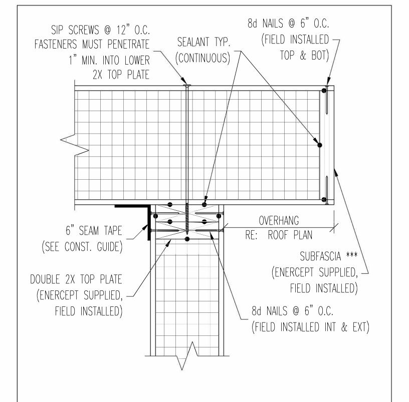
• WALL PANELS AT GABLE ENDS DO NOT RECEIVE A CAP PLATE OVER THE FULLY RECESSED TOP PLATES UNLESS NOTED OTHERWISE.
