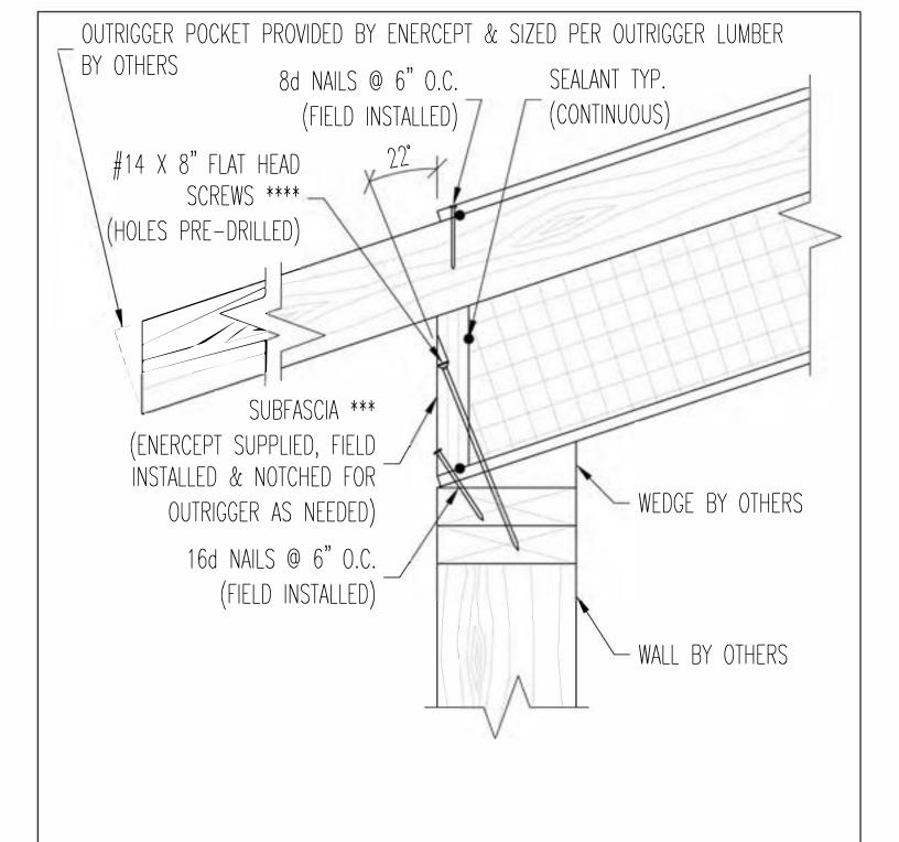
\*\*\* SUBFACIA INSTALLED IS BASED ON ROOF PANEL THICKNESS AND/OR STRUCTURAL REQUIREMENTS. ENERCEPT MAY INSTALL DIMENSIONAL 2X LUMBER, RIMBOARD, OR LVL.
