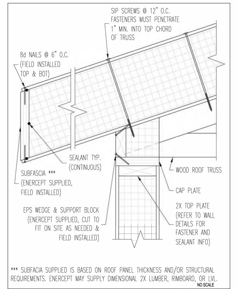
ROOF PANEL, PLUMB CUT, PANEL OVERHANG, TO WOOD ROOF TRUSS AT EAVE
