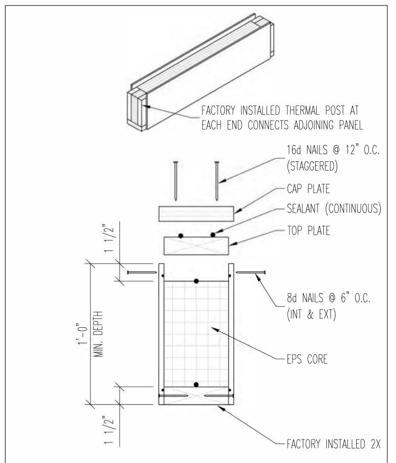
• DO NOT SPLICE TOP PLATE OR CAP PLATE OVER HEADER PANEL.
