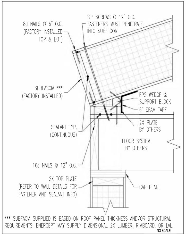
ROOF PANEL, SQUARE CUT, NO OVERHANG, FLOOR SYSTEM AT EAVE
