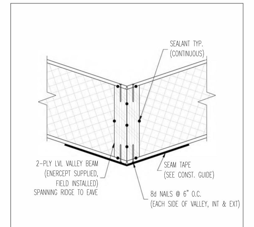
\* MULTI-PLY LUMBER TO BE GLUED, SEALED & NAILED TOGETHER AT FACTORY.
