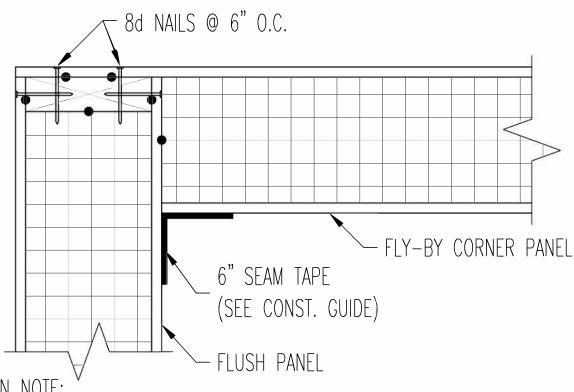
• A COME-A-LONG OR OTHER MECHANICAL MEANS MAY BE REQUIRED TO PULL PANELS TOGETHER.
