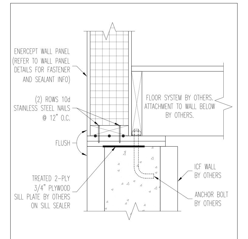
• THE BOTTOM PLATE SHALL BE SET IN A DISTANCE EQUIVALENT TO THE EXTERIOR SHEATHING THICKNESS. SQUARENESS AND ALIGNMENT OF THE BOTTOM PLATE ARE CRITICAL PARTS OF THE ENERCEPT SYSTEMS.
