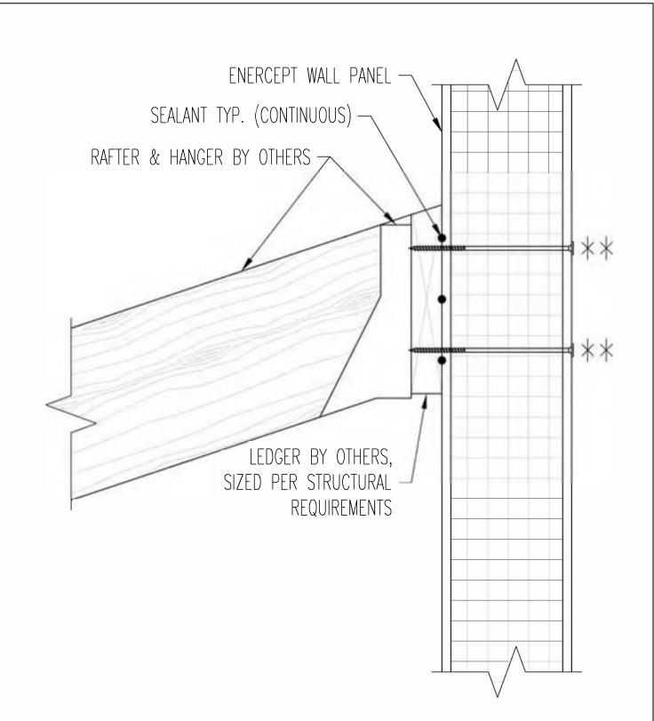
NOTE: ATTACHMENT OF LEDGER TO EXTERIOR OF WALL PANEL BY OTHERS.
