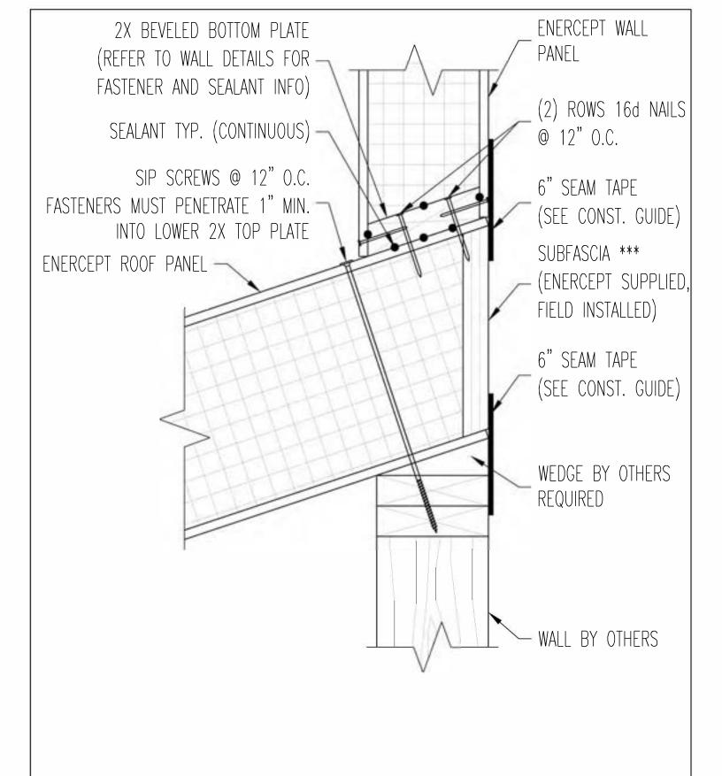
ROOF PANEL TO WALL BY OTHERS BELOW WALL PANEL ABOVE TO ROOF PANEL
