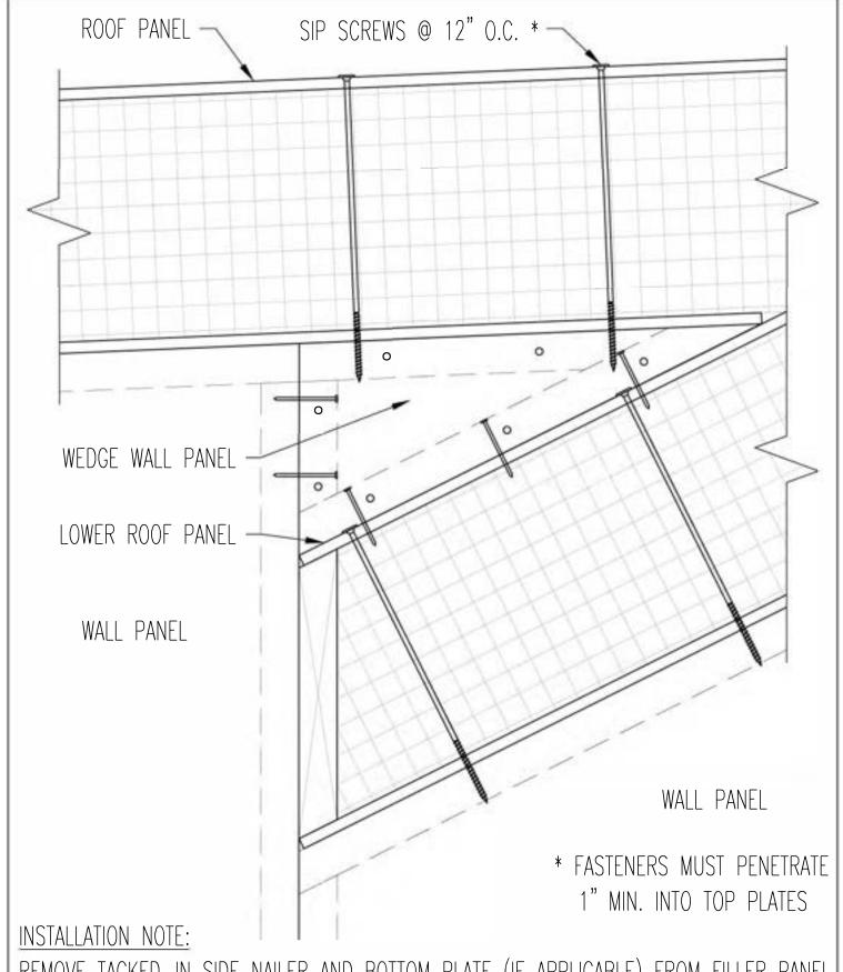
REMOVE TACKED-IN SIDE NAILER AND BOTTOM PLATE (IF APPLICABLE) FROM FILLER PANEL.
