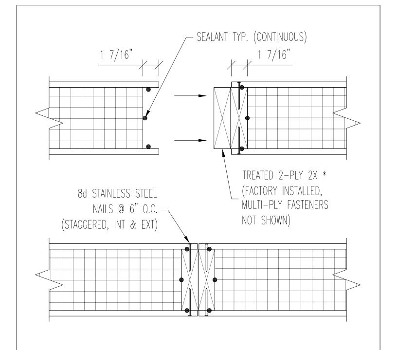
\* MULTI-PLY LUMBER TO BE GLUED, SEALED & NAILED TOGETHER AT FACTORY.
