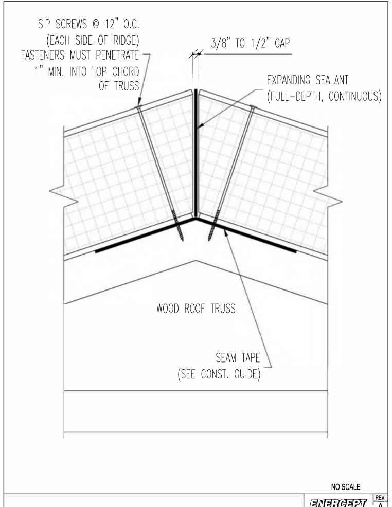
ROOF PANELS TO WOOD ROOF TRUSS AT RIDGE
