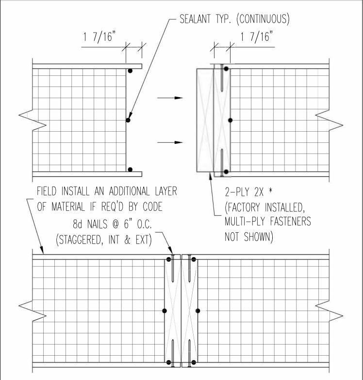
\* MULTI-PLY LUMBER TO BE GLUED, SEALED & NAILED TOGETHER AT FACTORY.
