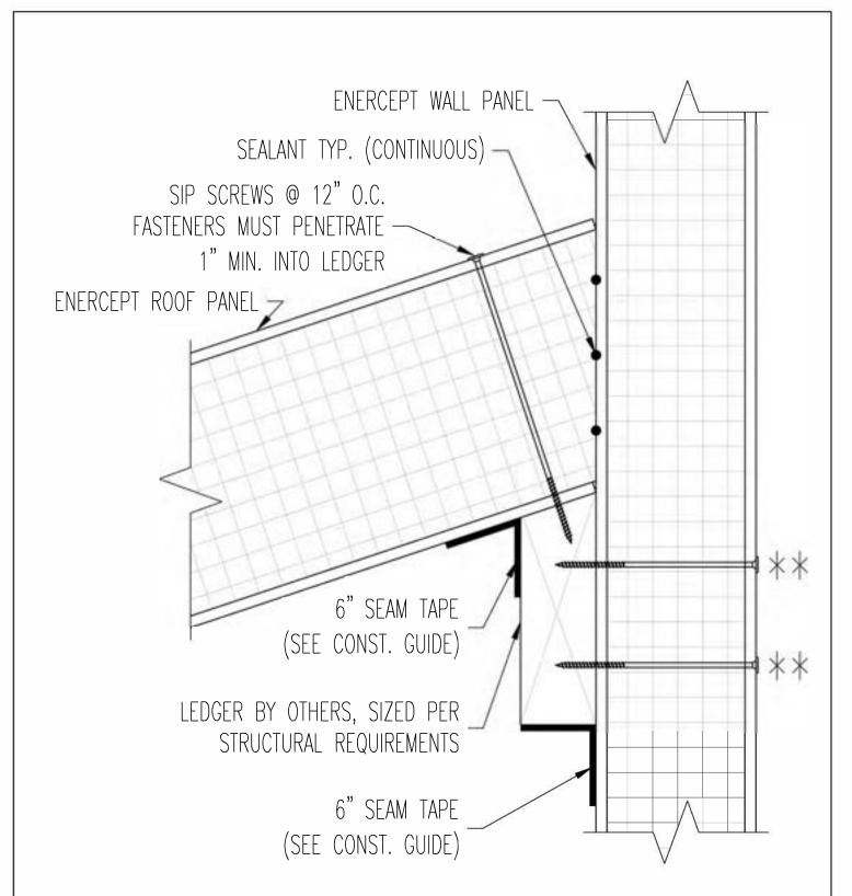
NOTE: ATTACHMENT OF LEDGER TO EXTERIOR OF WALL PANEL BY OTHERS.
