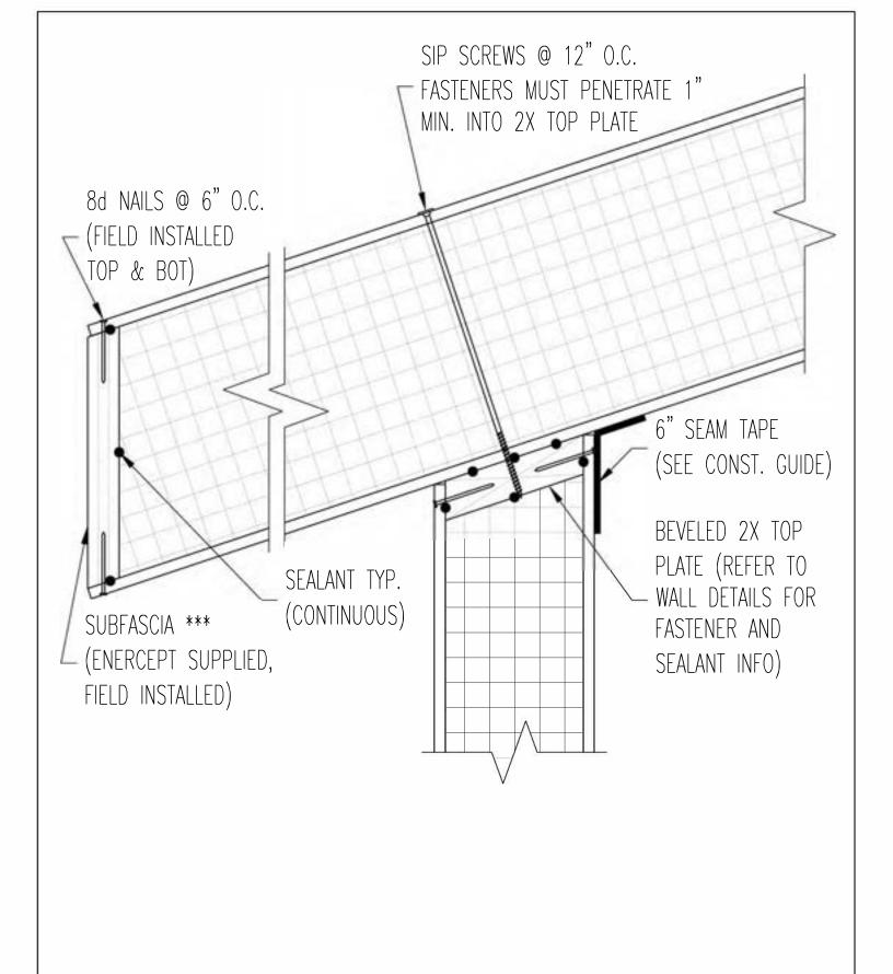
ROOF PANEL, PLUMB CUT, PANEL OVERHANG, BEVELED WALL PANEL AT EAVE
