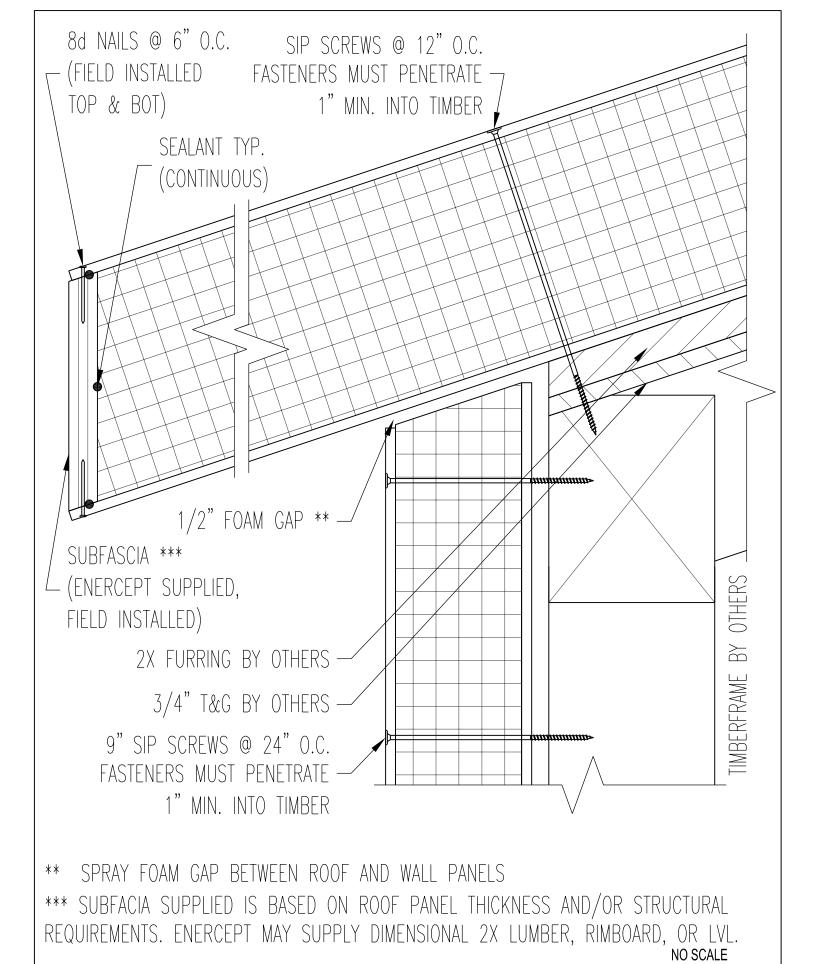
ROOF & WALL PANEL TO TIMBER FRAME AT EAVE, PLUMB CUT, PANEL OH, 2X FURRING & 3/4" T&G
