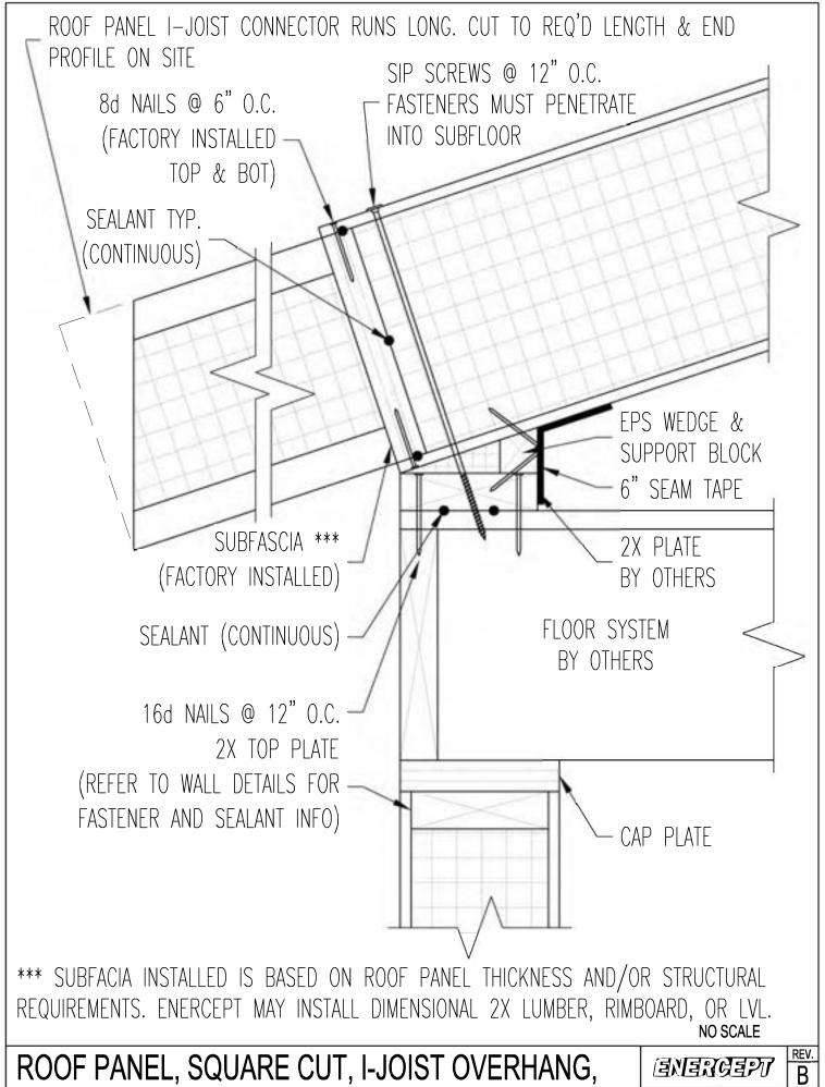
ROOF PANEL, SQUARE CUT, I-JOIST OVERHANG, FLOOR SYSTEM AT EAVE
