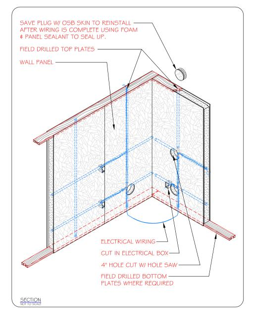
the default factory electrical chases are sufficient to provide adequate access for electrical runs; however, it would be best to review the SIP shop drawings¹ with your electrician and let your SIP manufacturer know if you would like to add any additional electrical chases within the SIPs.
